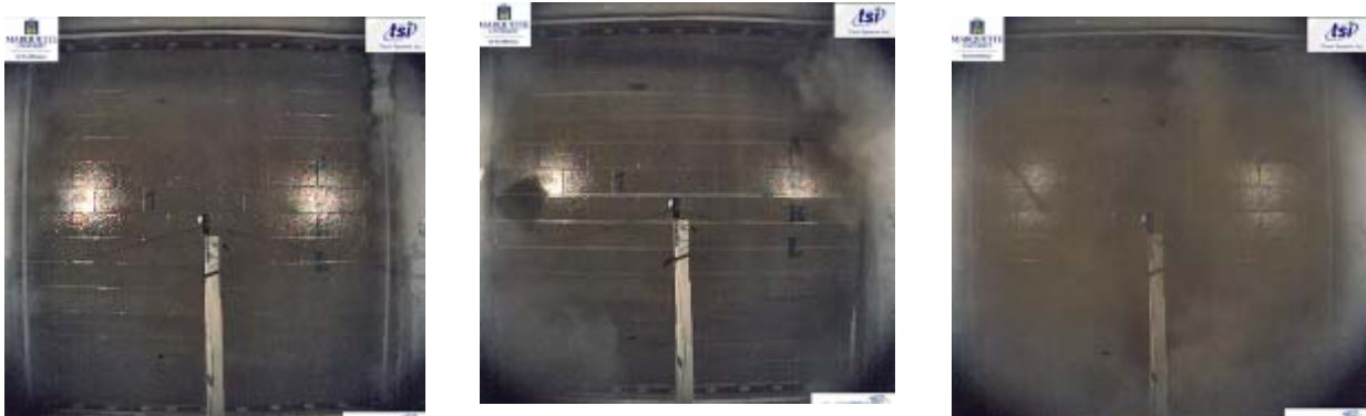
Walls with protective fire and blast coating deflect, but do not collapse.
